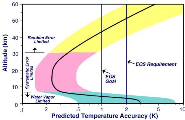
Fig. 2 Approximate occultation temperature accuracy vs altitude.
