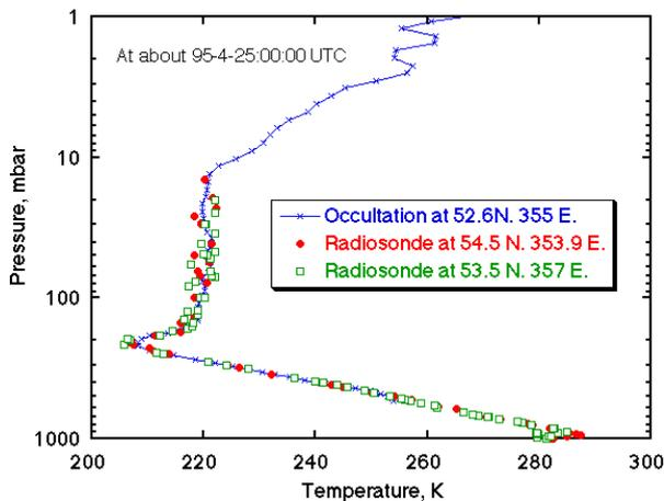
Fig. 3 GPS temperature profile compared with two radiosondes.
