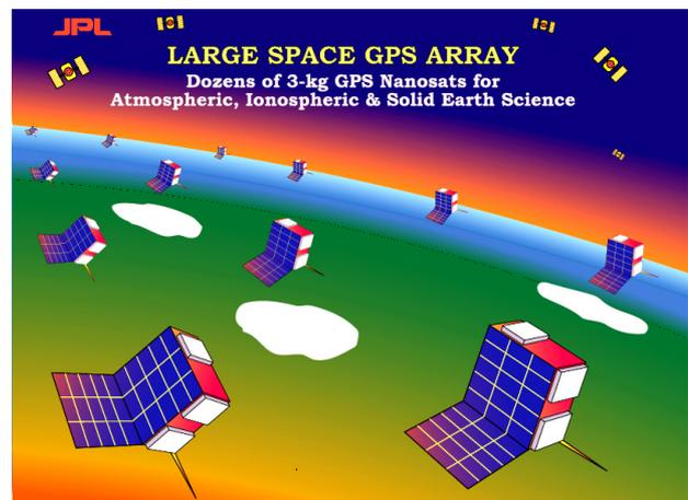
Fig. 4 Concept for a pilot constellation of spaceborne GPS sensorcraft for Earth science.
