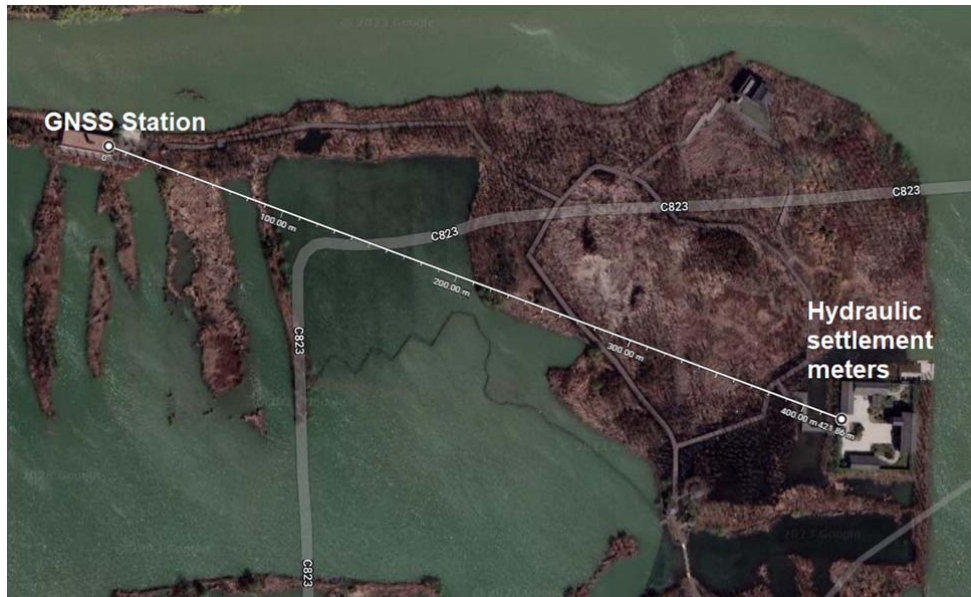
Fig. 2 Relative positions of the GNSS station and the hydraulic settlement meters
