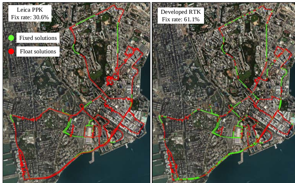
Fig. 7. Trajectories and fix rates of the two methods in Hong Kong
