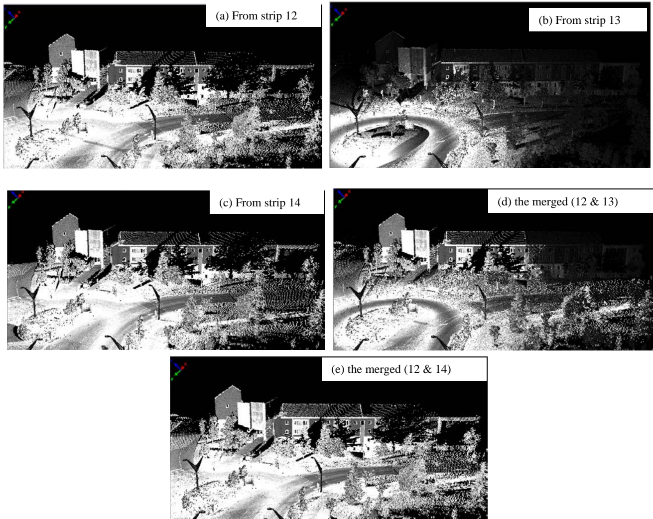
Fig. 17: An example of the merged patch: a LiDAR scanned scene around Calumet Resident (Area #1): (a) strip 12 (forward); (b) strip 13 (reverse), (c) strip 14 (forward), (d) the merged (strips 12 & 13) and (e) the merged (strips 12 & 14).
