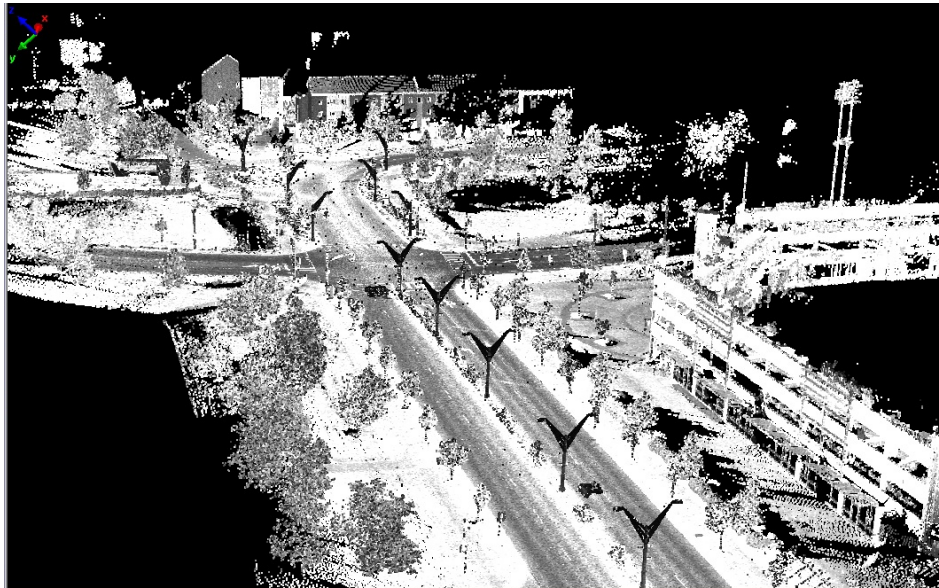
Fig. 6: Overview of Area #1 (Laser PRF:250kHz and mirror speed: 200Hz)
