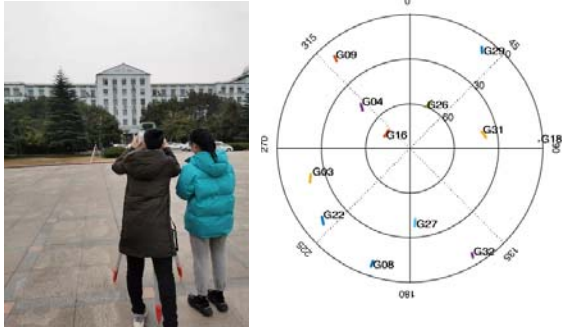
Figure 6 Experiment setup (left) and the skyplot of the tracked GNSS satellites (right)
