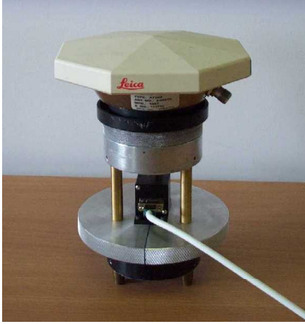
Fig. 8 A cage used to house a GPS antenna and a triaxial accelerometer
