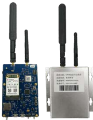
Fig.3 UWB anchor and tag two-in-one device
